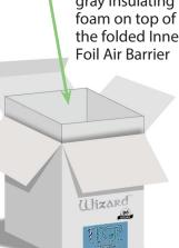
Finally, Fold the Outer Foil Air Barrier... Using a "gift wrap" fold... no need to glue or tape.
