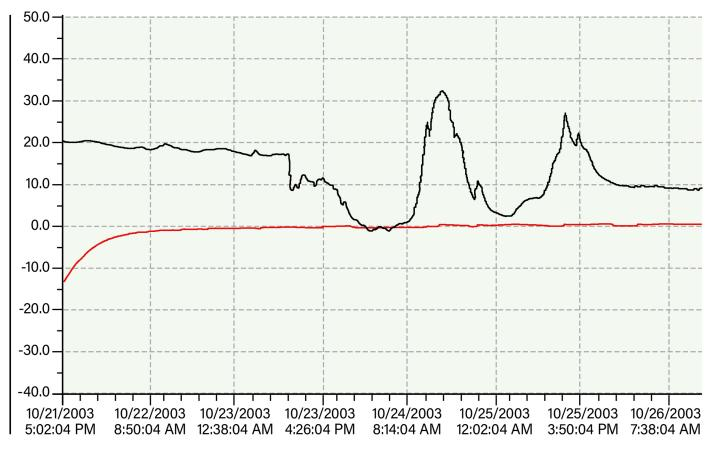
The **black** graph line represents the recorded outside temperatures during transit. The **red** graph line represents the recorded inside payload temperature during transit.
